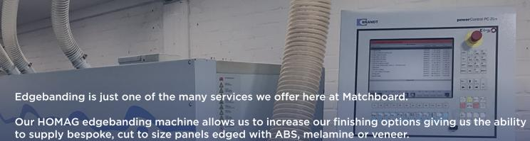
to supply bespoke, cut to size panels edged with ABS, melamine or veneer. It offers precise processing of coiled material to solid lipping's. Edge thickness from 0.4 to 3mm, panel thickness from 12 to 60mm. High quality edging to your sheet materials, the process is precise allowing for only a hairline join between edging.
