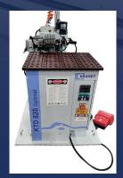
Our second edgebander, an Optimat KTD 820 is designed for shaped and curved work pieces. With direct glue application and vacuum table for clamping it can edge panels upto  $1m \times 1m$  with a band width of 20 to 45mm.
